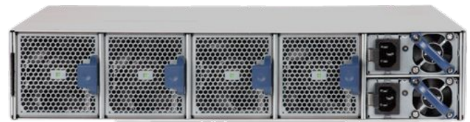
Arista 7250QX 2RU Rear View: Rear-to-front airflow model (blue)
